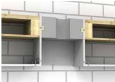
Wooden beam ceiling with classified ceiling substructure
