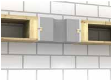
Wooden beam ceiling without ceiling substructure
